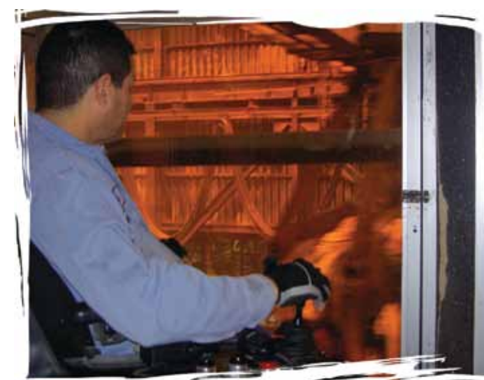
Above: Waste-to-energy plants help reduce the amount of waste. Here, a crane operator moves trash toward a furnace on the tipping floor about six stories below.
